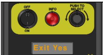
The control box will now display "Exit Yes" or by turning the "PUSH TO SELECT" knob anti clockwise "Exit No" Turning back will display "Exit Yes" again.
