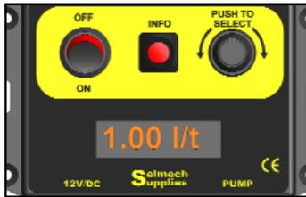
Press the "PUSH TO SELECT" knob to display the application rate in litres per tonne (l/t).
