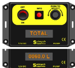
To clear the counter to zero, with the total litres displayed, press and hold the info button. After a few seconds the display will always revert to showing t/h
