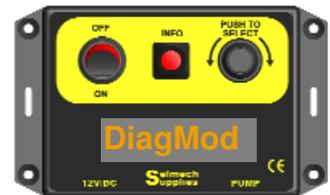
Press and release the “PRESS TO SELECT” as per diag mode but continue to hold until Diag++ is displayed.
