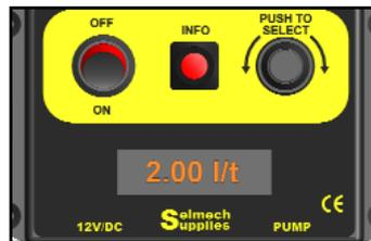
Press the "PUSH TO SELECT" knob again to display the application rate in l/t. Rotate the knob to set your application rate.
