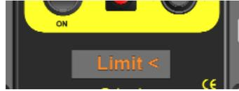
If the target flow is less than the specified minimum flow for the selected model the display shows - Limit <
