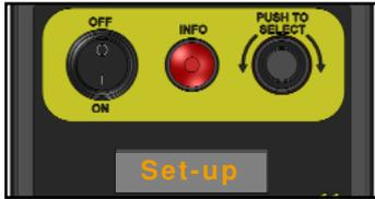
Keep holding down the "PUSH TO SELECT" Knob. The display will show "-----" then after about 10 seconds it will display "Set-up". Release the "PUSH TO SELECT" Knob.
